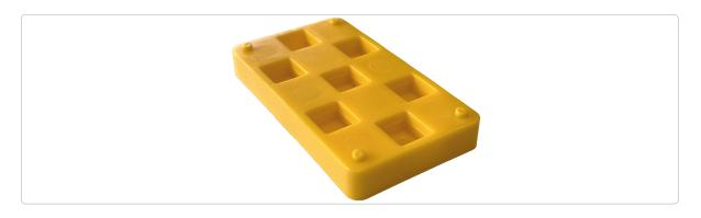
The K-Block 45C series has the same properties and functions as K-Block 45, but is simply in color-coded thicknesses. With its 45 mm, K-Block 45C is designed to accurately fit the width of rafters and other planed 2" wood, but is also used for distance adjustment and leveling of medium-heavy tasks such as doors and windows. The countersunk screw holes provide secure mounting.
